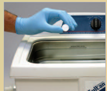
Pre-soak and disinfect instruments in an ultrasonic cleaner or soaking tray prior to terminal sterilization
