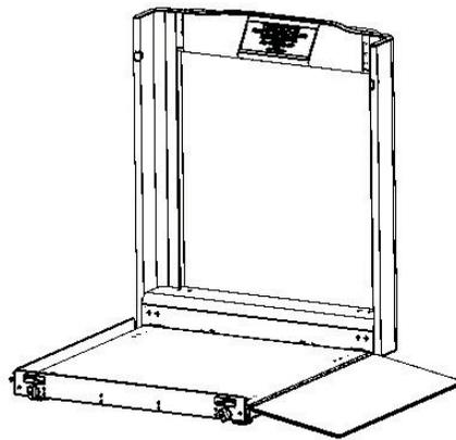
9. To close the scale you MUST turn both knobs counterclockwise on the lower back of the scale base.
