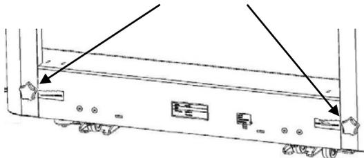
7. Push and turn knob until tight by hand clockwise to lock. Turn counterclockwise to release.
