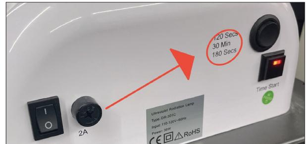
**7** Place the object in the Asiga Flash cure box with the base of the object flat on the tray. Set a timer to 12 minutes. On the Asiga Flash, press “time start” to begin curing. At this time, start your 12 minute timer.
